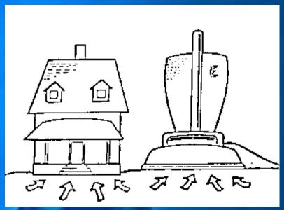
Air pressure differentials between the building and outside air causes radon from the soil to be drawn into the house resulting in elevated indoor radon levels.
